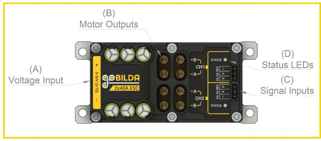
**(A) Voltage Input:** The ESC requires a DC input voltage between 9 and 30V. Choose a voltage that is appropriate for the motors you plan to use with the controller. The power input port is an XT90 connector that supplies power to both channels. This power input is reverse-polarity protected up to -30V.
