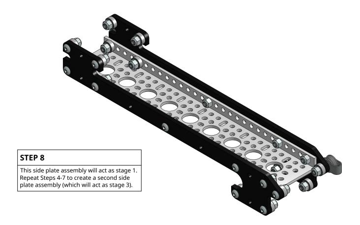
Using a 9-hole channel, create the assembly shown below.
