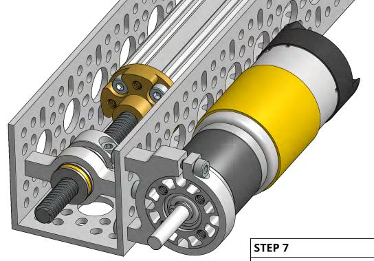
Insert a motor into the clamping mount as shown. Tighten the pinch bolt. This kit does not include a motor; a 5202-0002-0005 is shown as an example.
