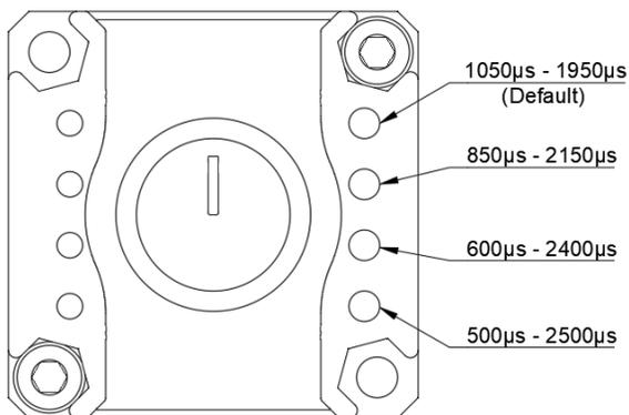
**1050µs-1950µs** is the default PWM range. This range allows most servos to rotate 90 degrees. Many servos are able to rotate further, given a wider range. If you purchased a goBILDA® Servo, reference the servo page for the maximum PWM range the servo is able to accept, and the corresponding rotation. This range is also used with goBILDA linear servos.
